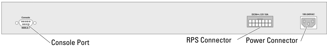
Figure 2-2. PowerConnect 3524 Back Panel
